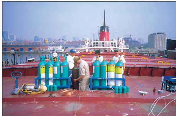
The set up of ECO 2 FUME™ cylinders for one of the phosphine treatments.
