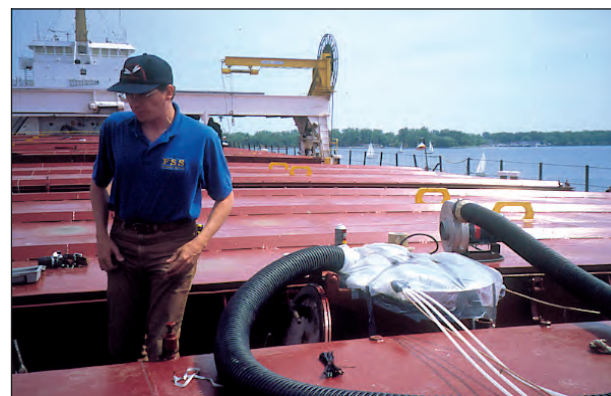
Pressure testing the seals of the ship holds prior to fumigation
